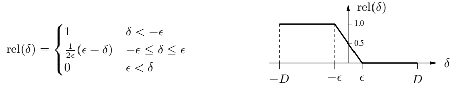
Fig. 1. The definition of the relational function \text{rel}() and its plot which maps the grey scale difference \delta to [0, 1] . D denotes the maximum grey scale value.
