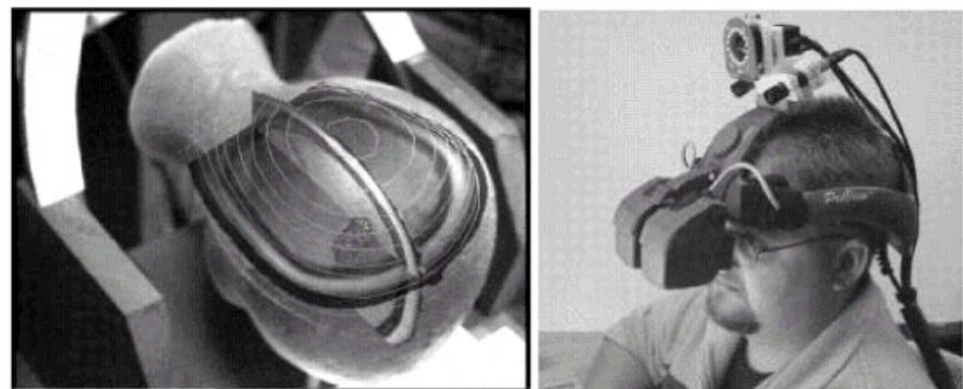
Fig. 5. Left image: video view of head phantom augmented with skull contour lines and the model of a tumor, segmented from a set of magnetic resonance (MR) images. Two of the MR slices are also shown. Right image: Video-see-through head-mounted display with additional tracker camera.
