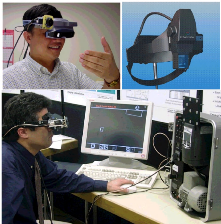
Fig. 4. The various components of our see-through system. A Sony XC-55BB camera with an infra-red filter is attached to one of the head-mounted displays (the video see-through display from Mixed Reality Labs and the two optical see-through devices the Virtual Retinal Scan Display (VRD) from Microvision and the I-glasses. The attached camera observes a set of retro-reflective markers for tracking. The camera is surrounded by a set of infra-red LEDs to illuminate the scene for optimal real-time tracking.
