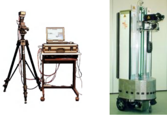
Fig. 1. Tripod and mobile acquisition robot (Autonomous Environmental Sensor for Telepresence AEST [9]).
