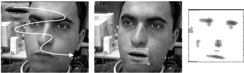
Fig. 2. Searching for the lips, left the searched pattern, middle the pattern matched, right regions where \rho > \text{threshold} .
